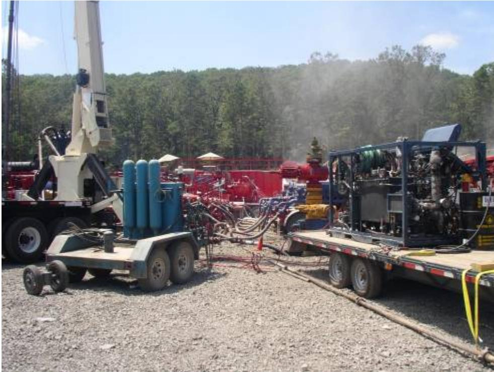
Figure 16 - The well being fraced is behind the white crane. The other wellhead near the middle of the picture was fraced on the previous day. In this case, two wells were constructed at the same well pad.
