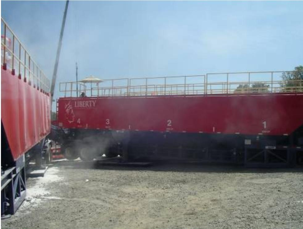
Figure 14 – Sand storage tanks.
