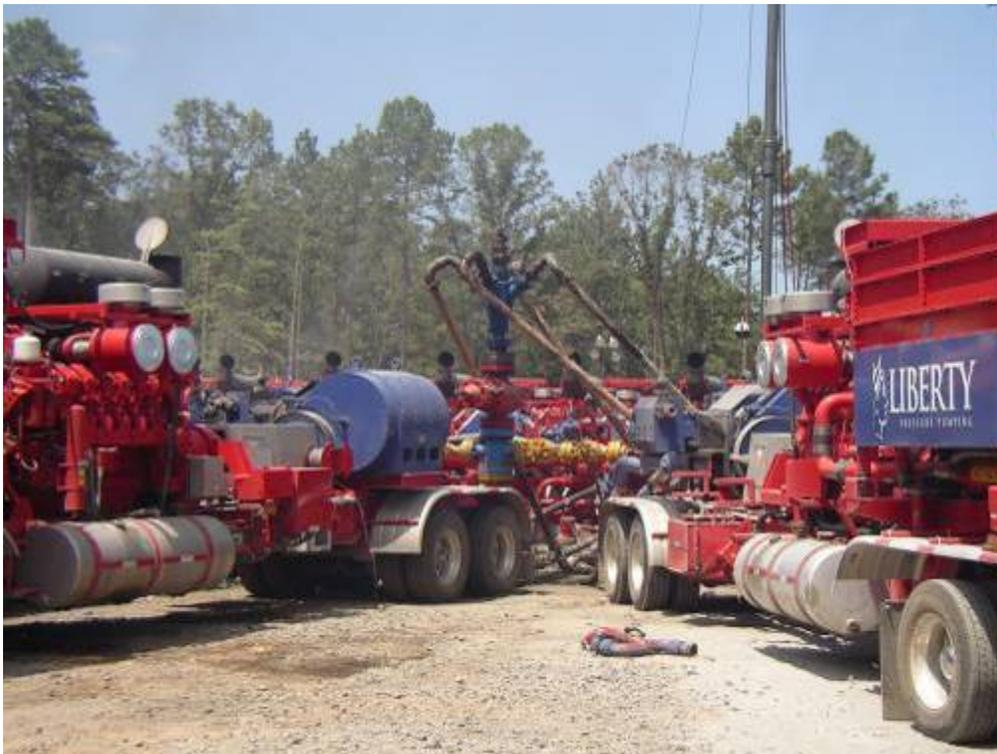
Figure 15 – The well being fraced is in the middle, with the pipe conveying the injectate. The two trucks beside the well are pumping units.
