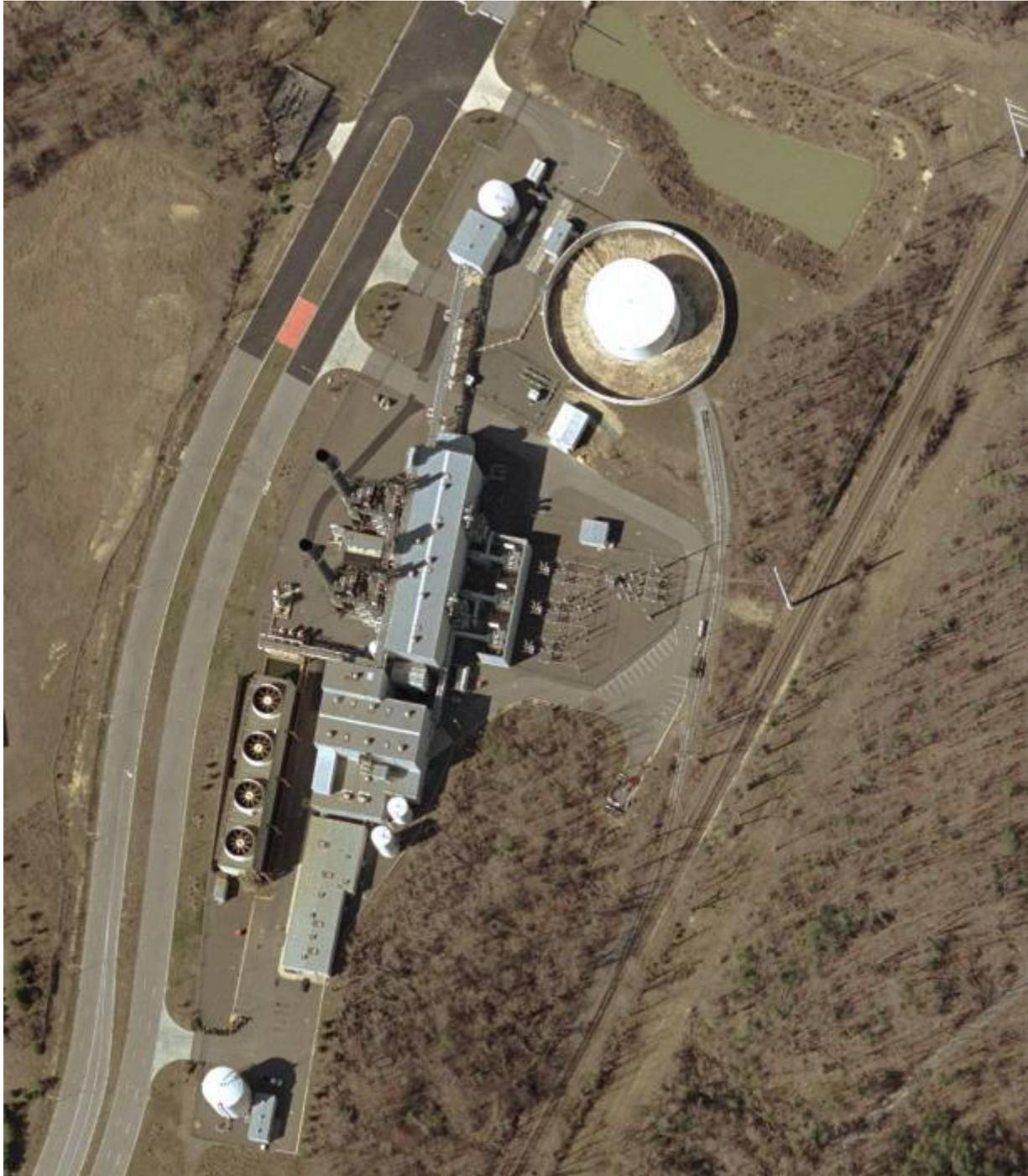
The plant began production in October 1996. The plant is a natural gas-fired combined-cycle plant with two combustion turbines and two heat recovery steam generators. It has a capacity of 230 MW. Number 2 distillate oil (stored in the large round tank seen in the upper right corner of Figure 3) is used as a back-up fuel for a limited number of hours each year.
